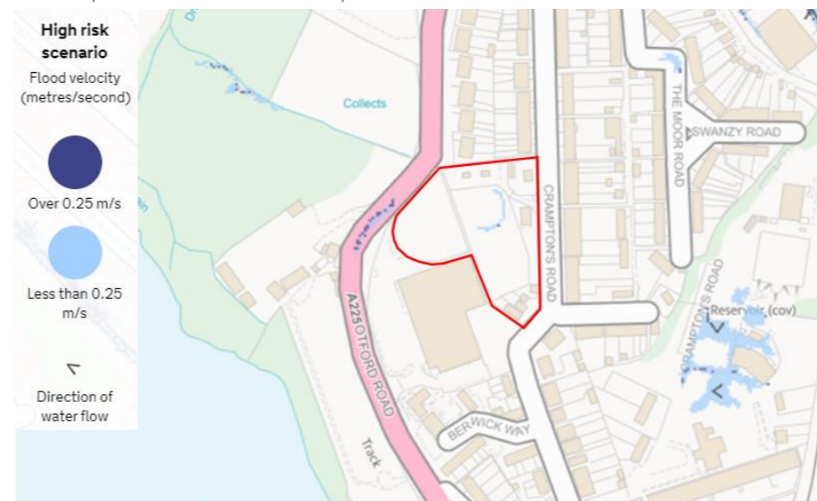
Flood Map for Surface Water Runoff Velocity
