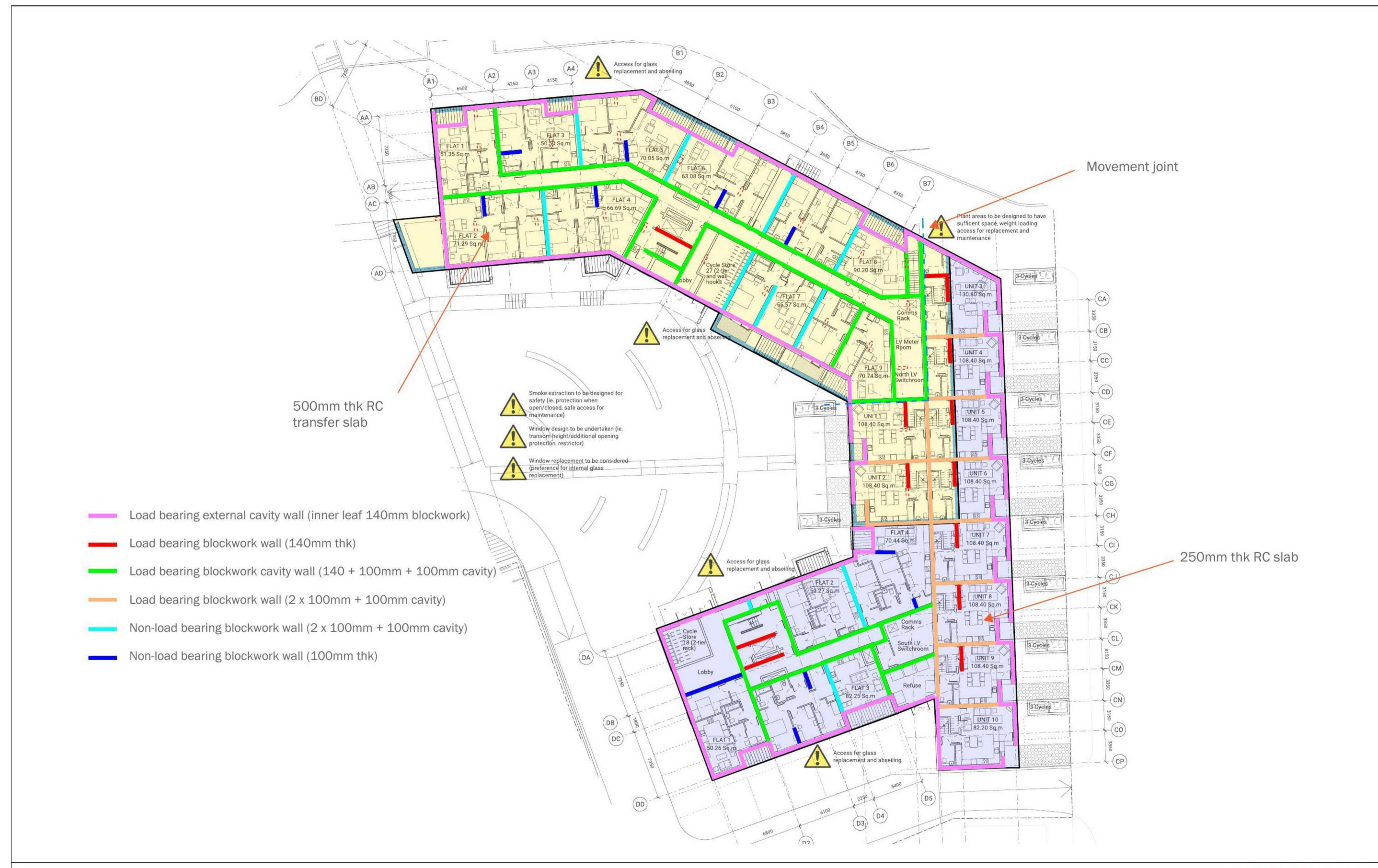
Main Building - Masonry + Precast Ground Floor (L00)
