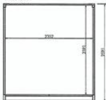
20ft Shipping Container - Section
