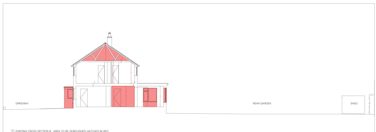
① EXISTING CROSS SECTION B AREA TO BE DEMOLISHED HATCHED IN RED
