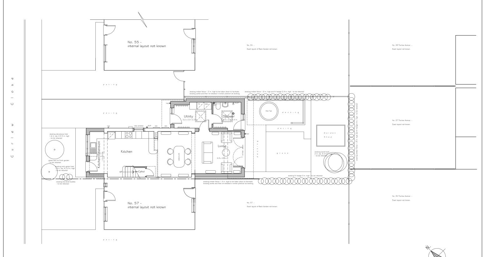
SITE PLAN AS PROPOSED - INCLUDING PROPOSED GROUND FLOOR PLAN.
