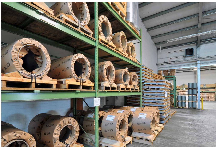
Storage of coils with wooden sleepers
