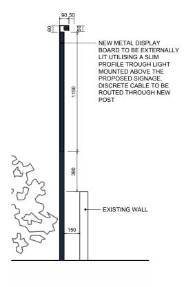
DETAILED SIGNAGE SIDE ELEVATION 1:25 @ A3
