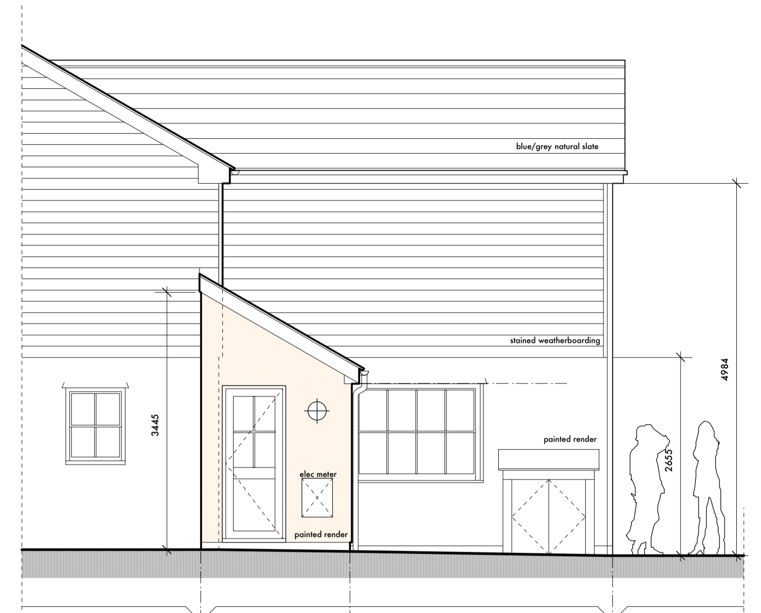
Existing Side Elevation (south-west) 1:50
