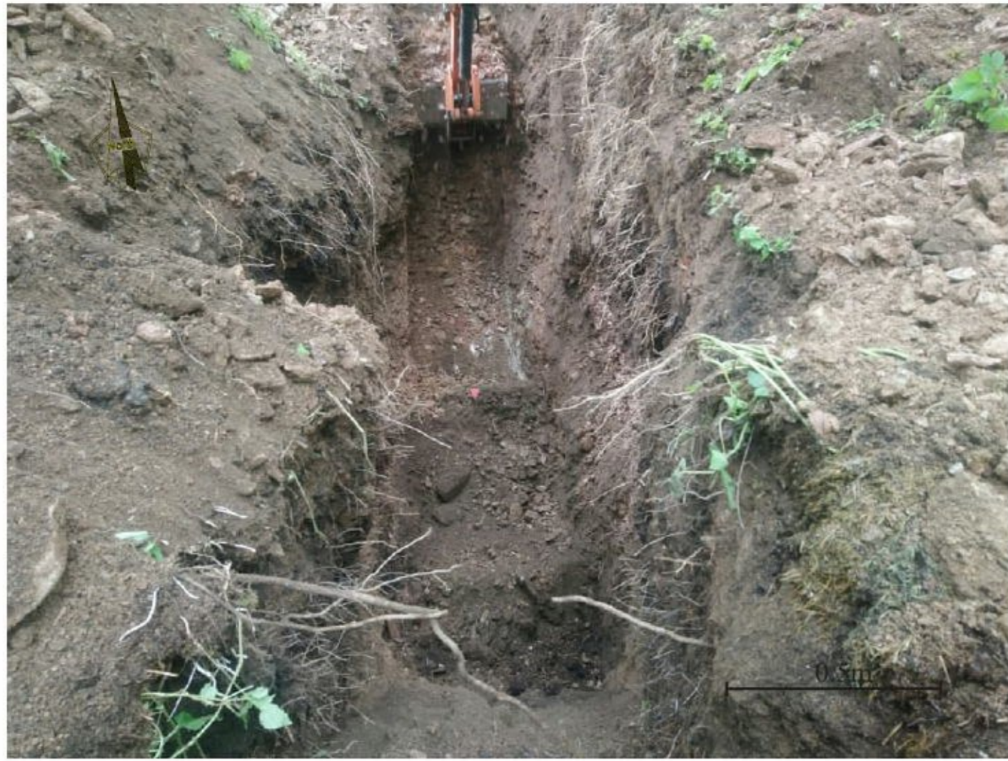
Photograph 1. In-situ weathered and fresher rock, overlain by stony clay and soil horizons, inferred to indicate northern limits of quarry.
