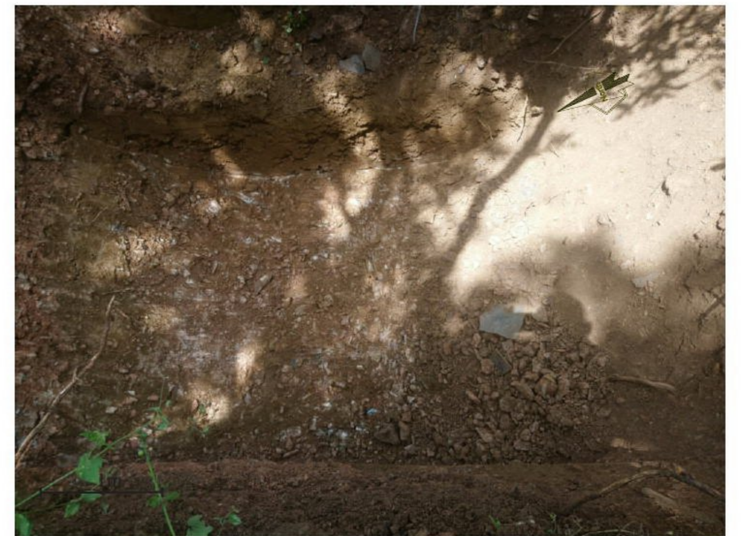
Photograph 6. In-situ stony clay encountered in position of suspected shaft, adjacent to northwestern.
