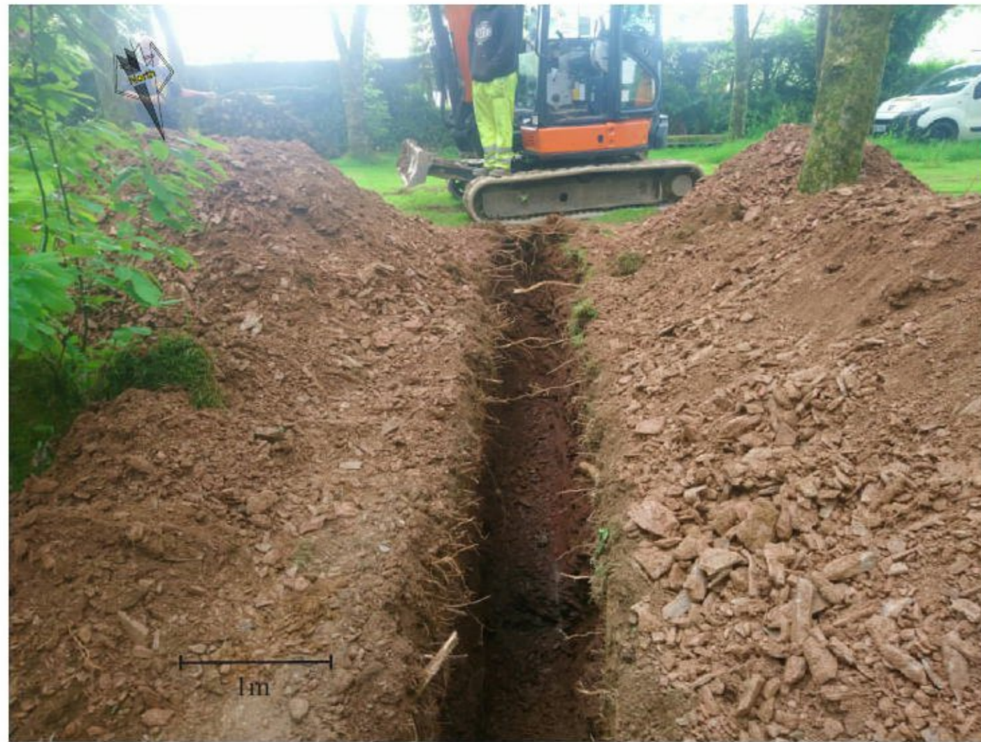
Photograph 4 View looking south along central trench showing consistency of encountered fill horizons comprising angular cobbles of metasediments with interstitial pink/buff clays.
