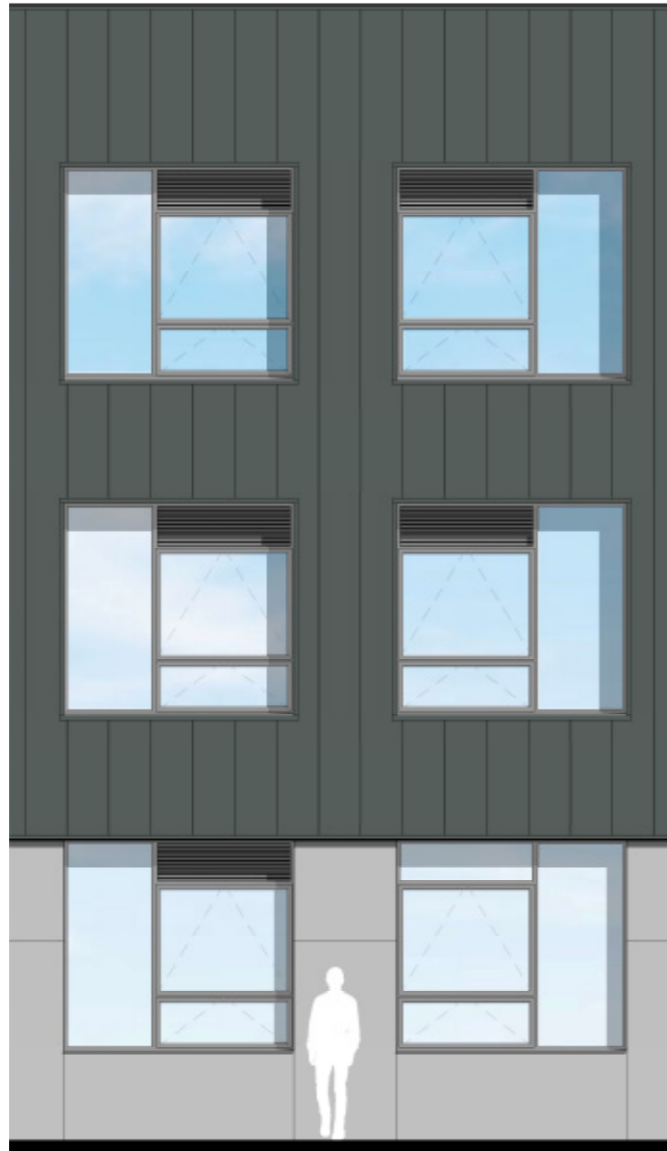
Merlin grey aluminium raised seam with grey fibre cement paneling
