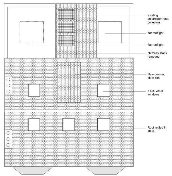
$1 \quad \frac{\text{Loft Plan}}{\text{Scale: 1:100}}$
