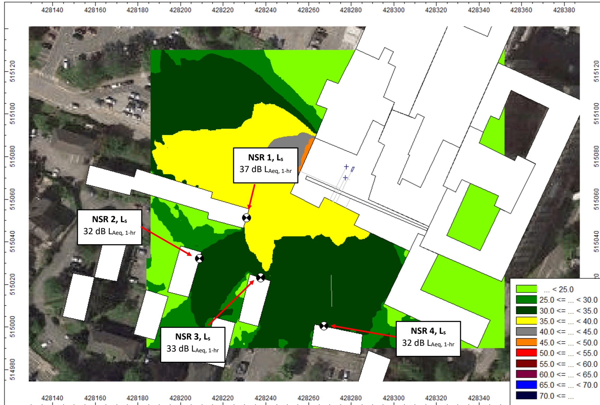
Figure 3: Sound contours at 4 m, showing the calculated specific sound level, LAeq,1 hr based on current proposals
