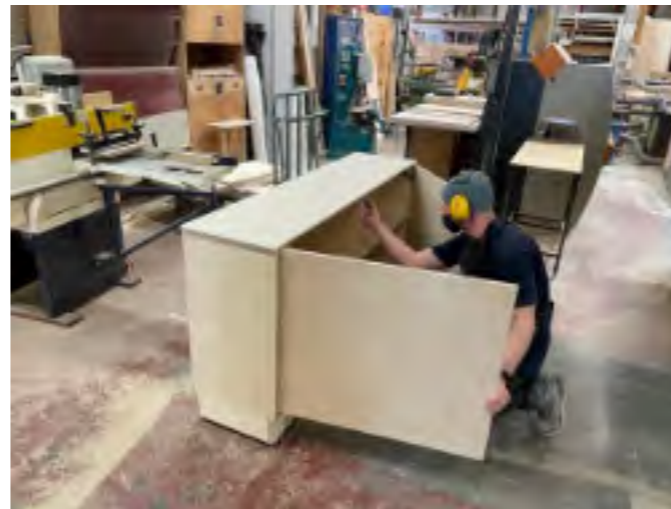
Example of cabinet fabricated and assembled in workshop
