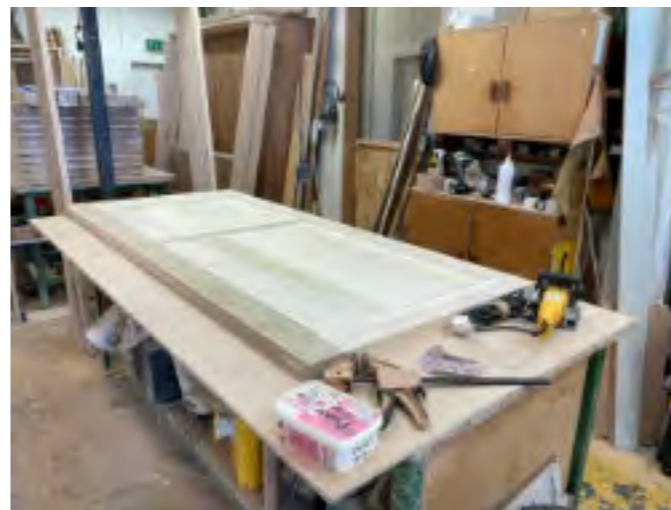
Example of panelled door fabricated and assembled in workshop
