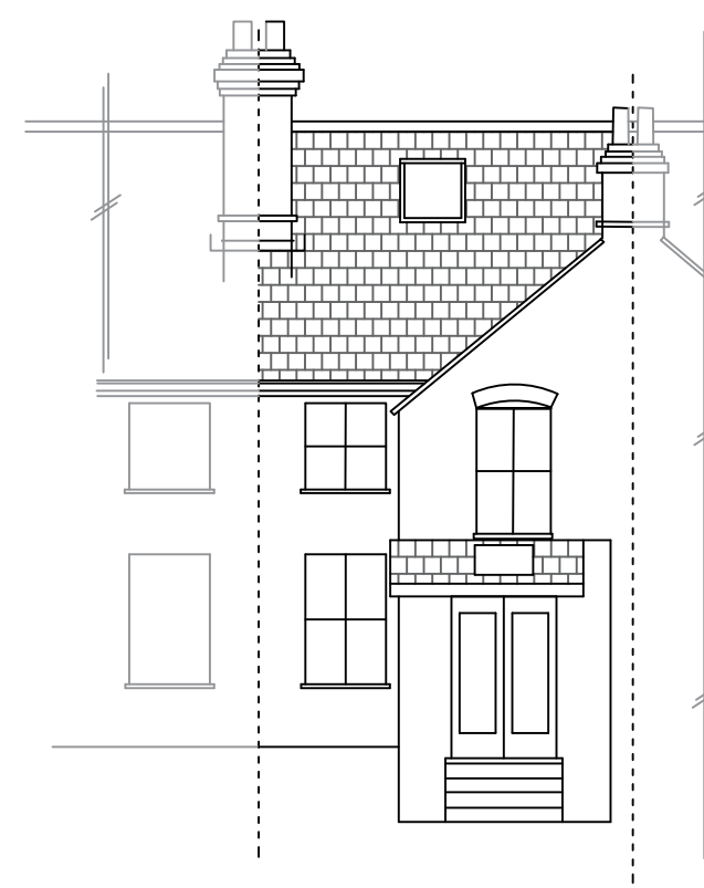
Existing rear elevation
