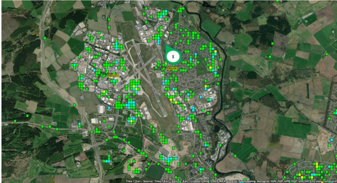
Figure 1 – Coverage Plots showing the required area to be covered showing the best location from a coverage perspective – needs to be as close as possible to green marker.
