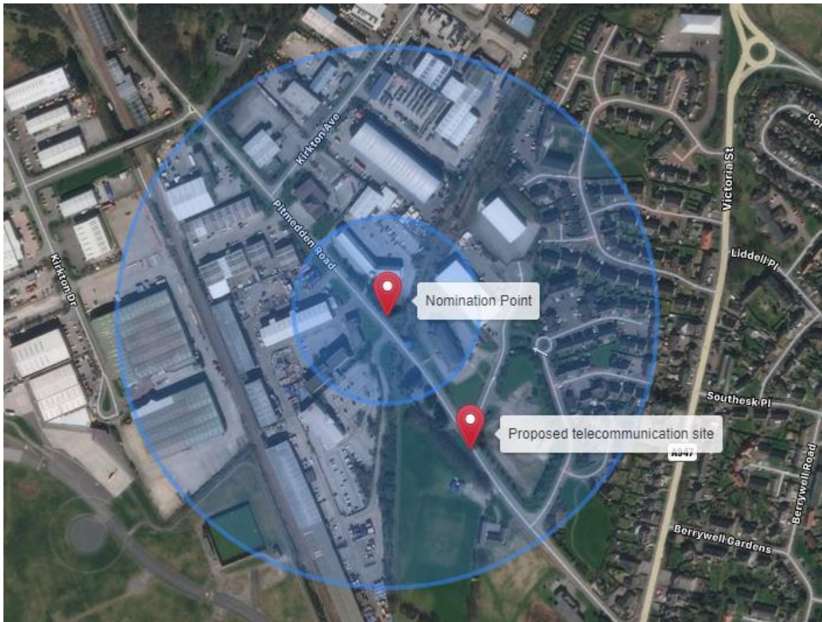
Figure 2 – Search area shown on aerial view for proposed new telecommunications mast – note that the proposed site normally requires be within 100 metres of the Nominal location for mast
