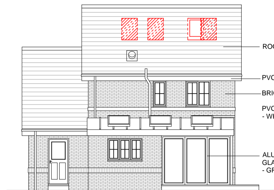
Existing North West Elevation, Scale 1:100
