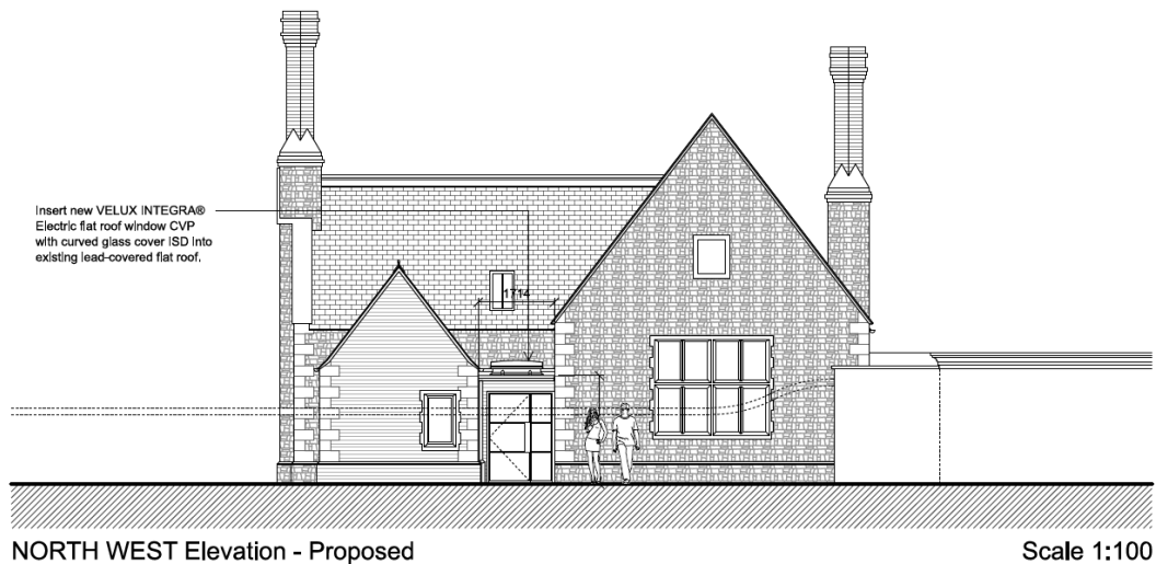
Proposed roof window insertion in flat roof as seen on proposed elevation drawing.
