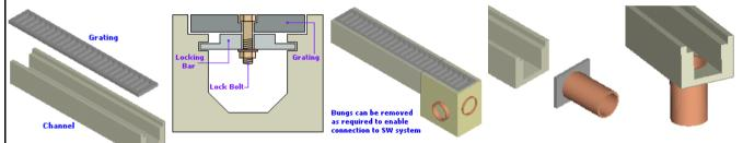
**Above**; Illustrations showing typical linear surface water drainage system components with from the left; an expanded view of a complete section, a grate fixing detail, a 'silt-box' type connection, a pipe union end cap and bottom outlet connections
