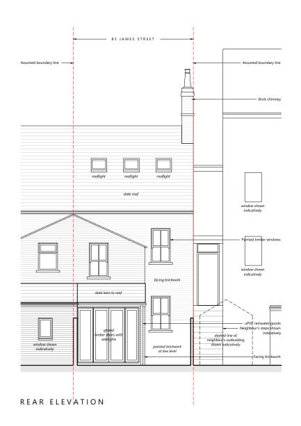
Do not scale from this drawing. All dimensions are approximate and should be checked on site prior to construction.
