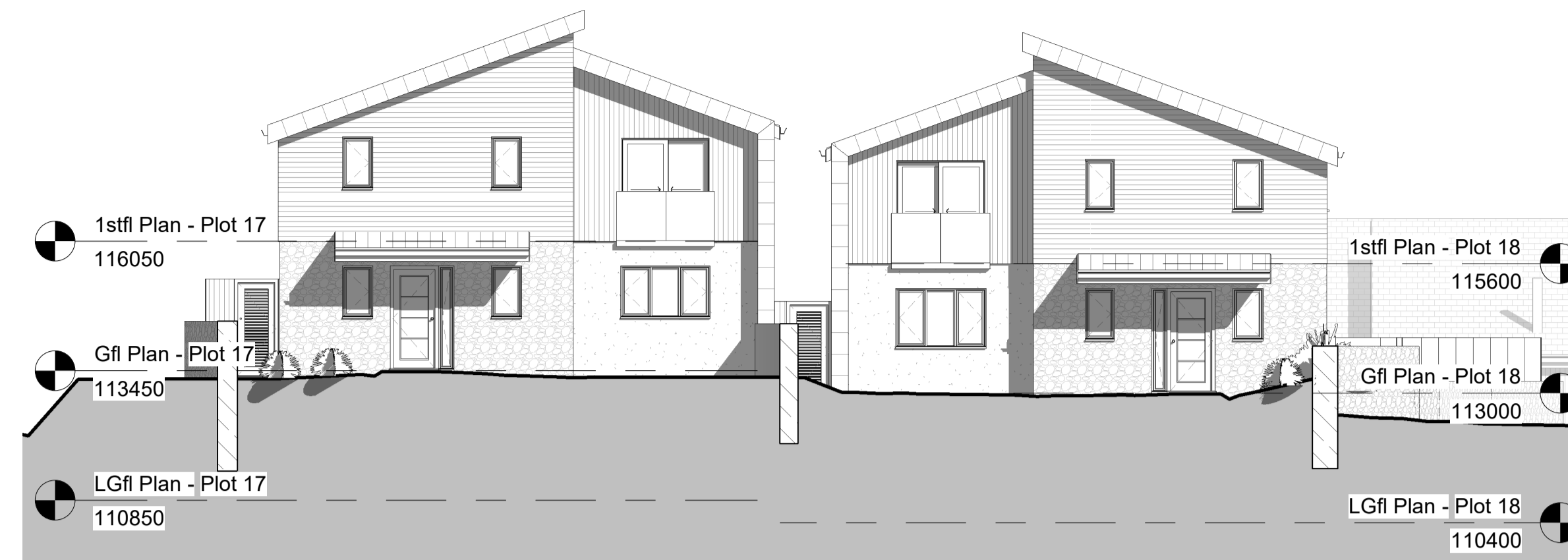
1 West Elevation - Plots 17 & 18 1 : 100
