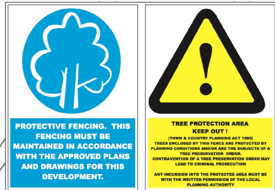
Protective Barrier Fencing - Example Design
