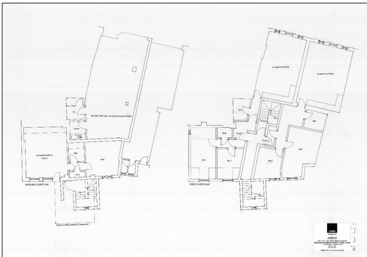
Fig 6: Proposed ground and first floor layout plans (Reproduced by courtesy of CHESS Architecture & Development Limited)
