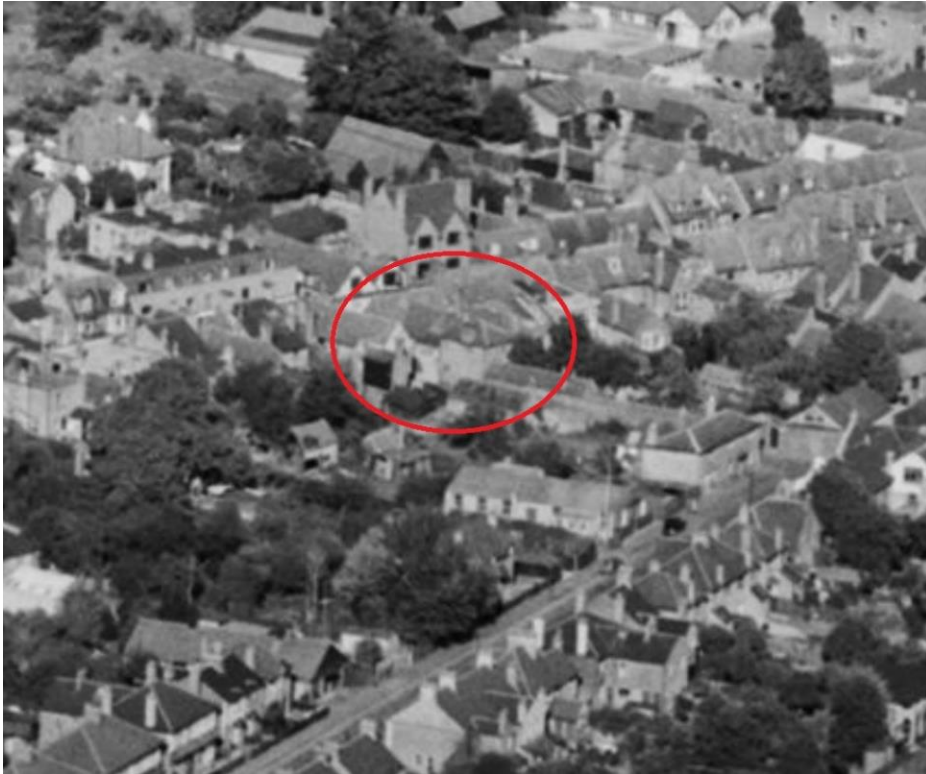
Fig. 5: Extract from oblique aerial photograph (1949) looking SW and showing the L-shaped extension to the rear of Nos. 129-131 and No. 133 High Street Rickmansworth, with double hipped roof (circled in red) (Reproduced by courtesy of the Historic England Archive)
