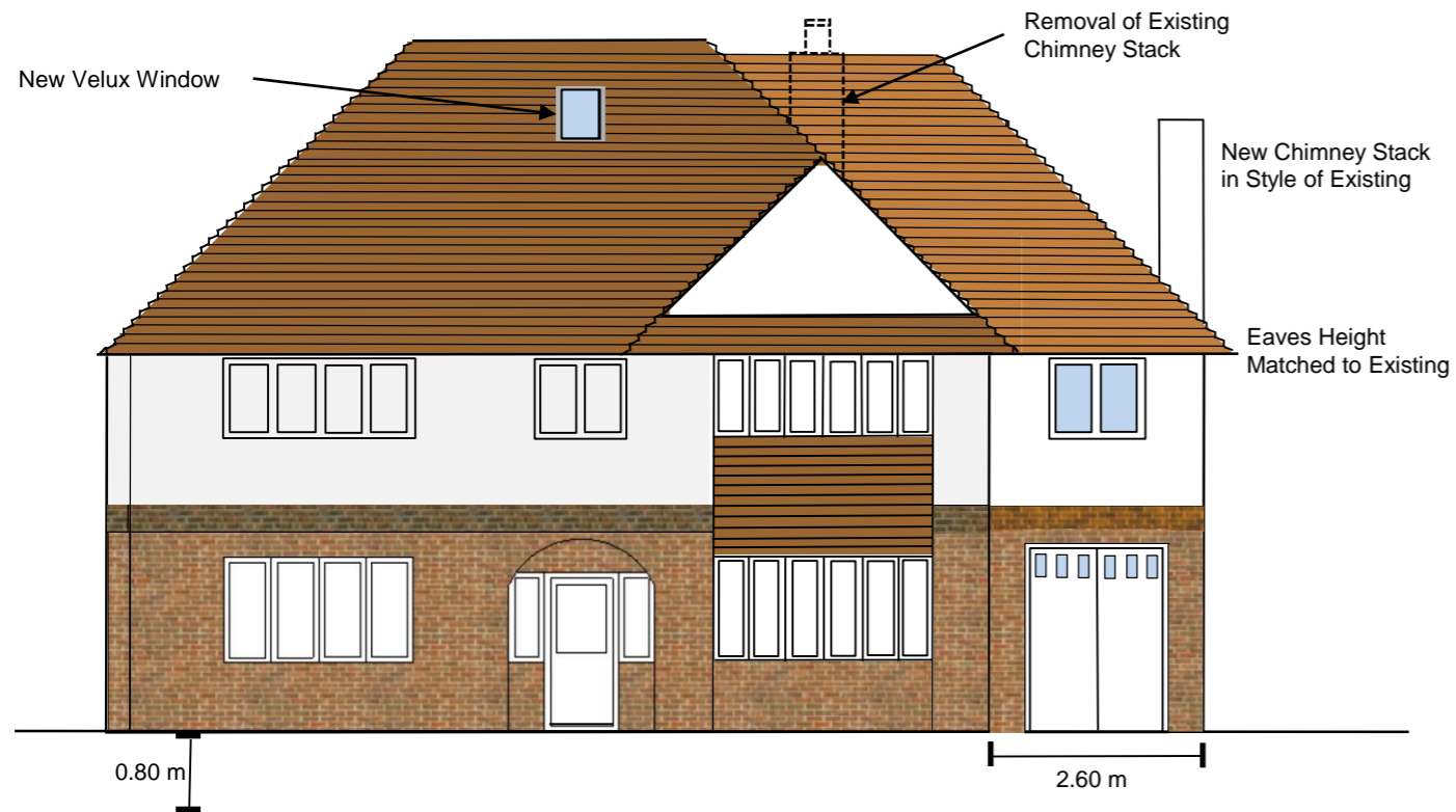
FRONT ELEVATION (SOUTH EAST)
