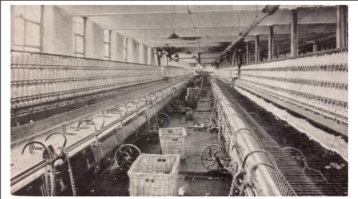
Figure 17 –One of the mule spinning rooms, driven by electricity (now all removed) (Source: Illustrated London News – 10 th July 1909)
