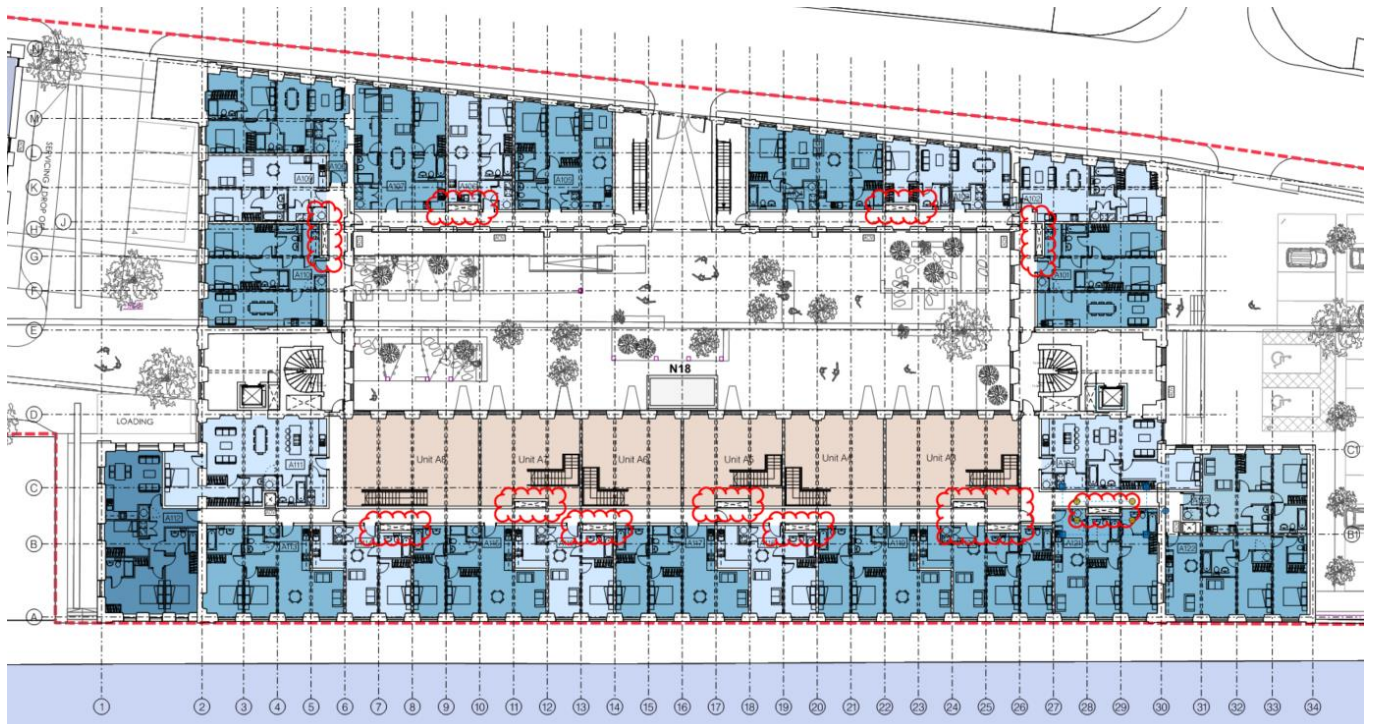
Mill building apartment mechanical ventilation risers to accommodate fresh air inlet and exhaust air ductwork from ground floor to roof.
