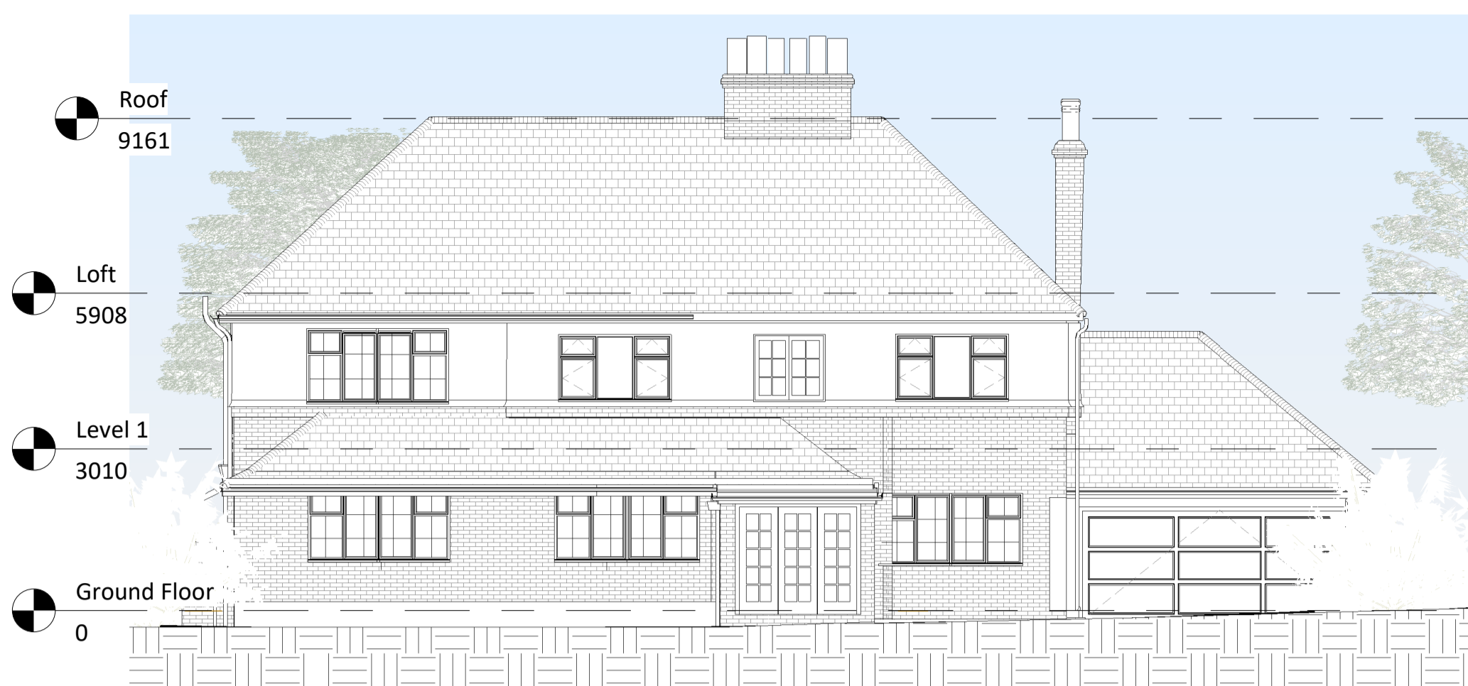
3 Existing Front Elevation 1 : 100
