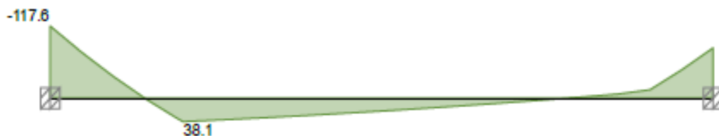
Strength combinations - Moment envelope (kNm)
