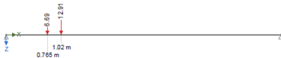
Imposed - Loading (kN)
