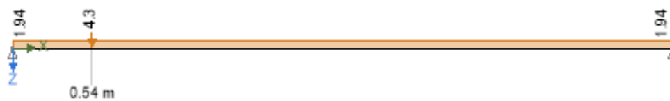
Permanent - Loading (kN/m,kN)
