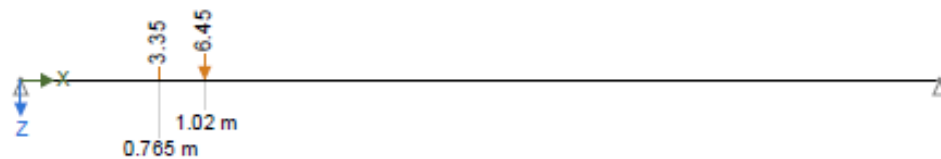
Permanent - Loading (kN)
