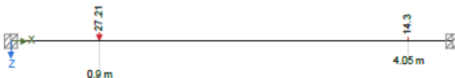
Imposed - Loading (kN)
