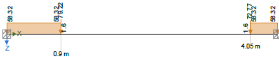
Permanent - Loading (kN/m,kN)
