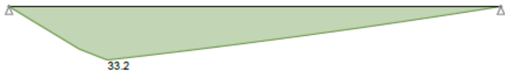
Strength combinations - Moment envelope (kNm)
