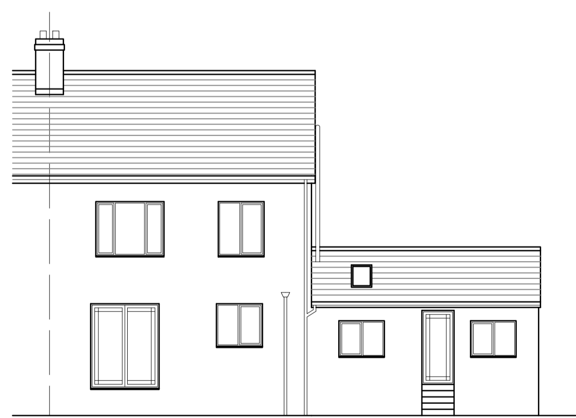
Rear Elevation as Existing 1:100
