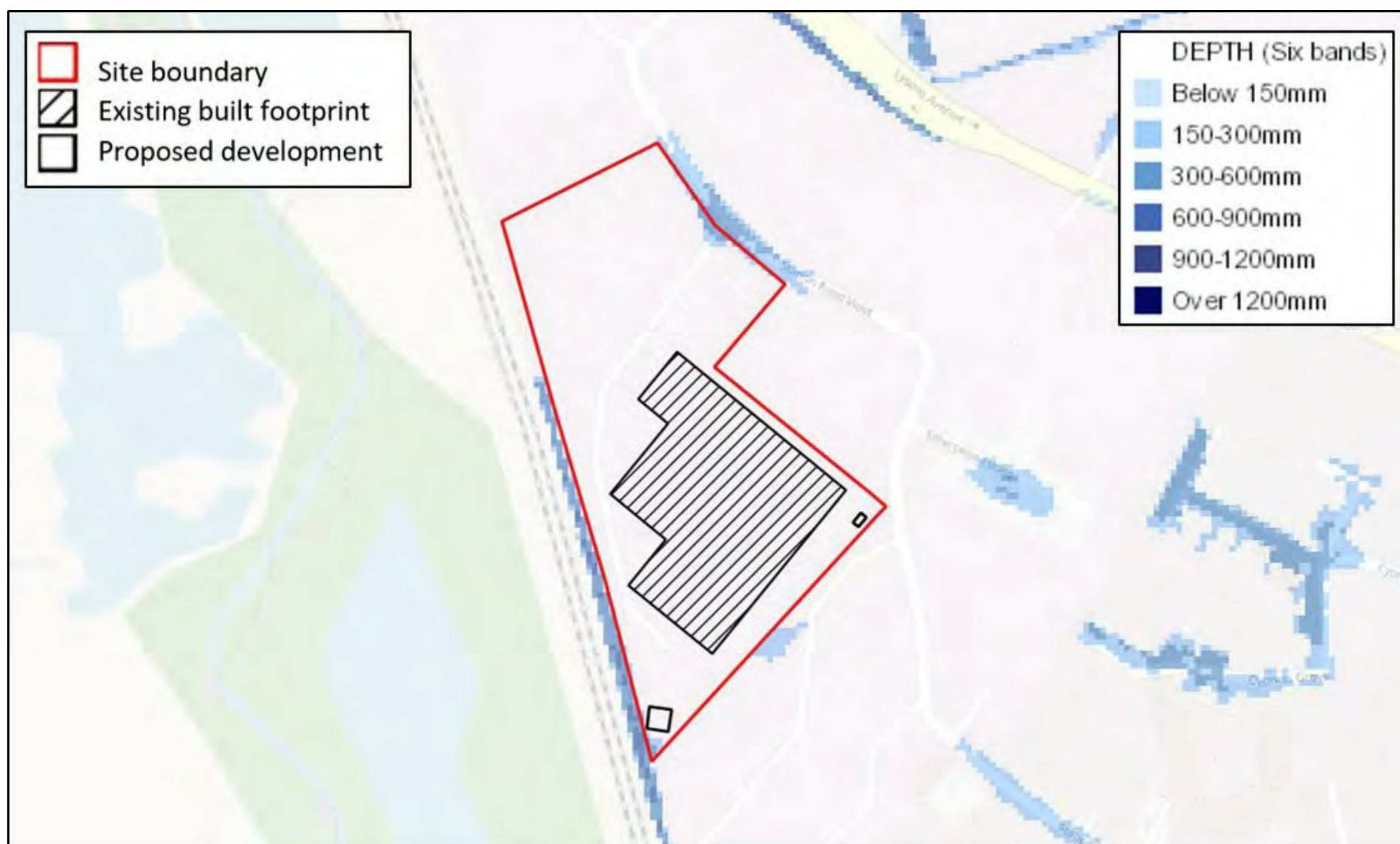
Figure 10: EA modelled 1:100-year surface water event, showing location of site (Source: EA)
