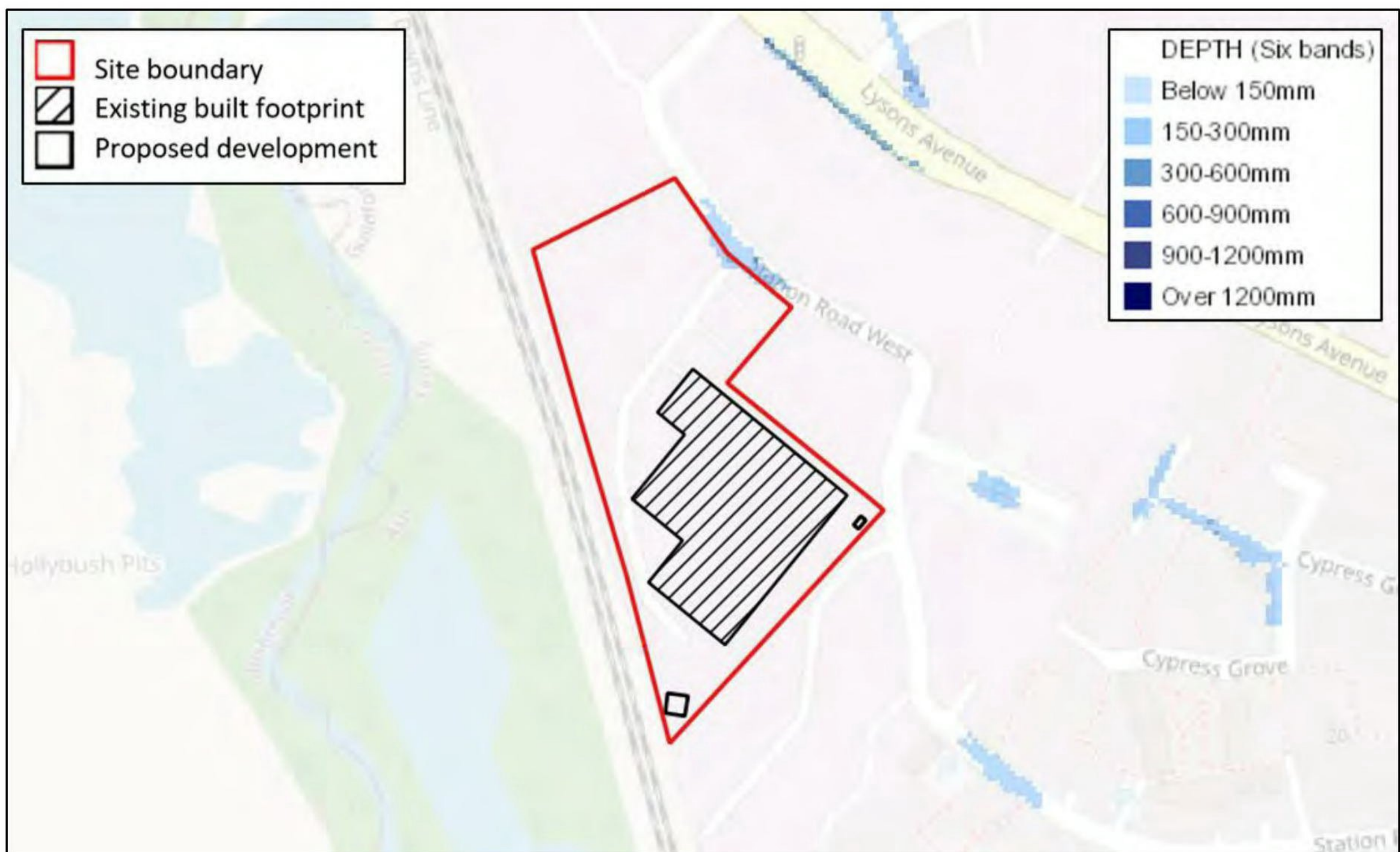
Figure 9: EA modelled 1:30-year surface water event, showing location of site (Source: EA)
