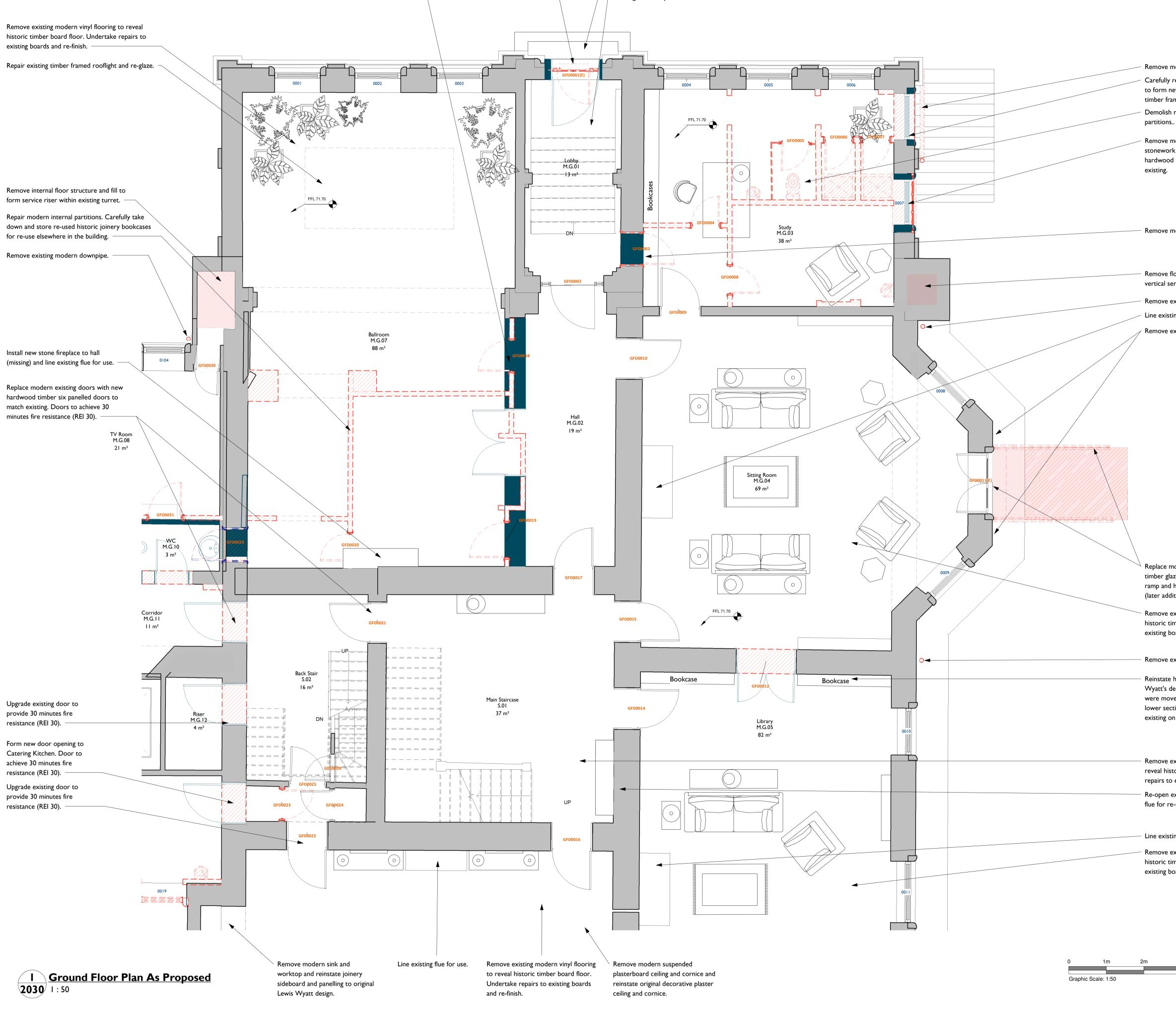
Drop external level to reveal bottom steps to Lewis Wyatt's original design.
