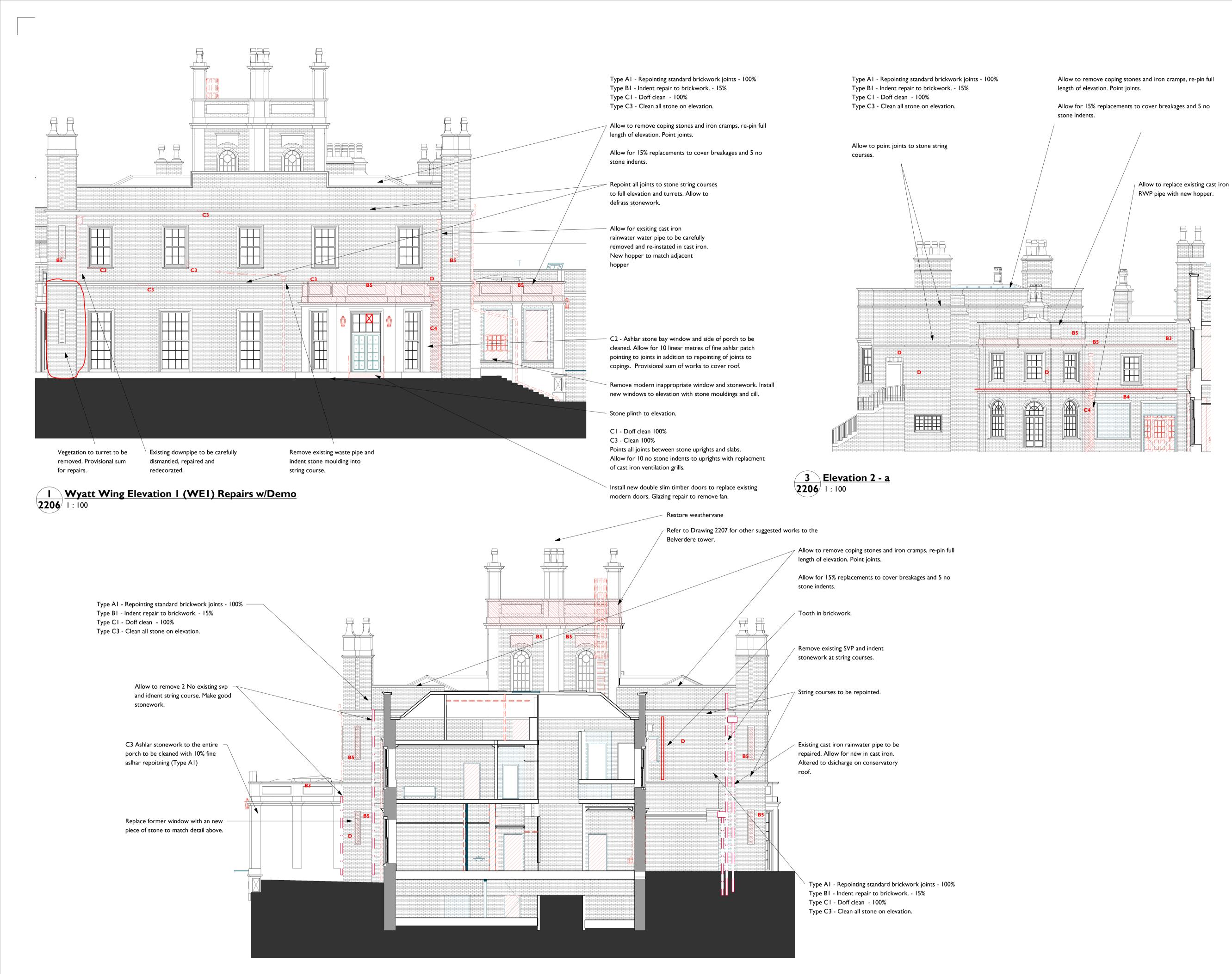
2 Wyatt Wing Elevation 2 (WE2) Repairs w/Demo **2206** 1 : 100
