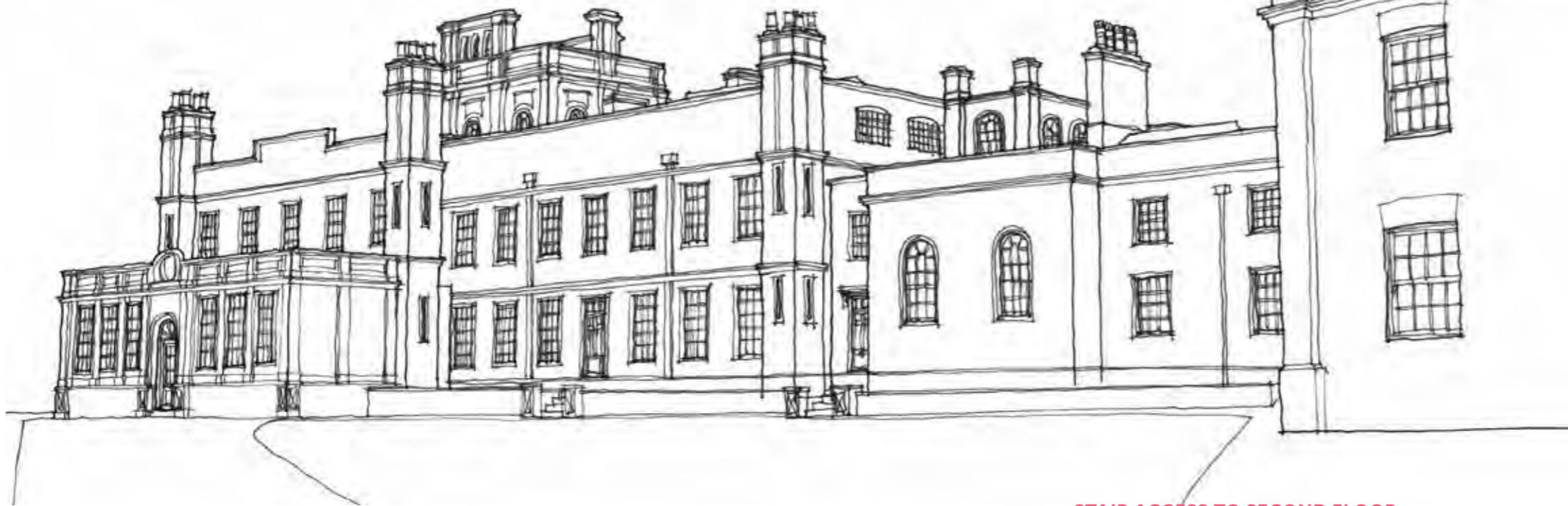
Above: Sketch view of Cuerden Hall as proposed from the entrance drive, showing the proposed stair enclosure at second floor level to gain access to the existing second floor of the 1717 House.
