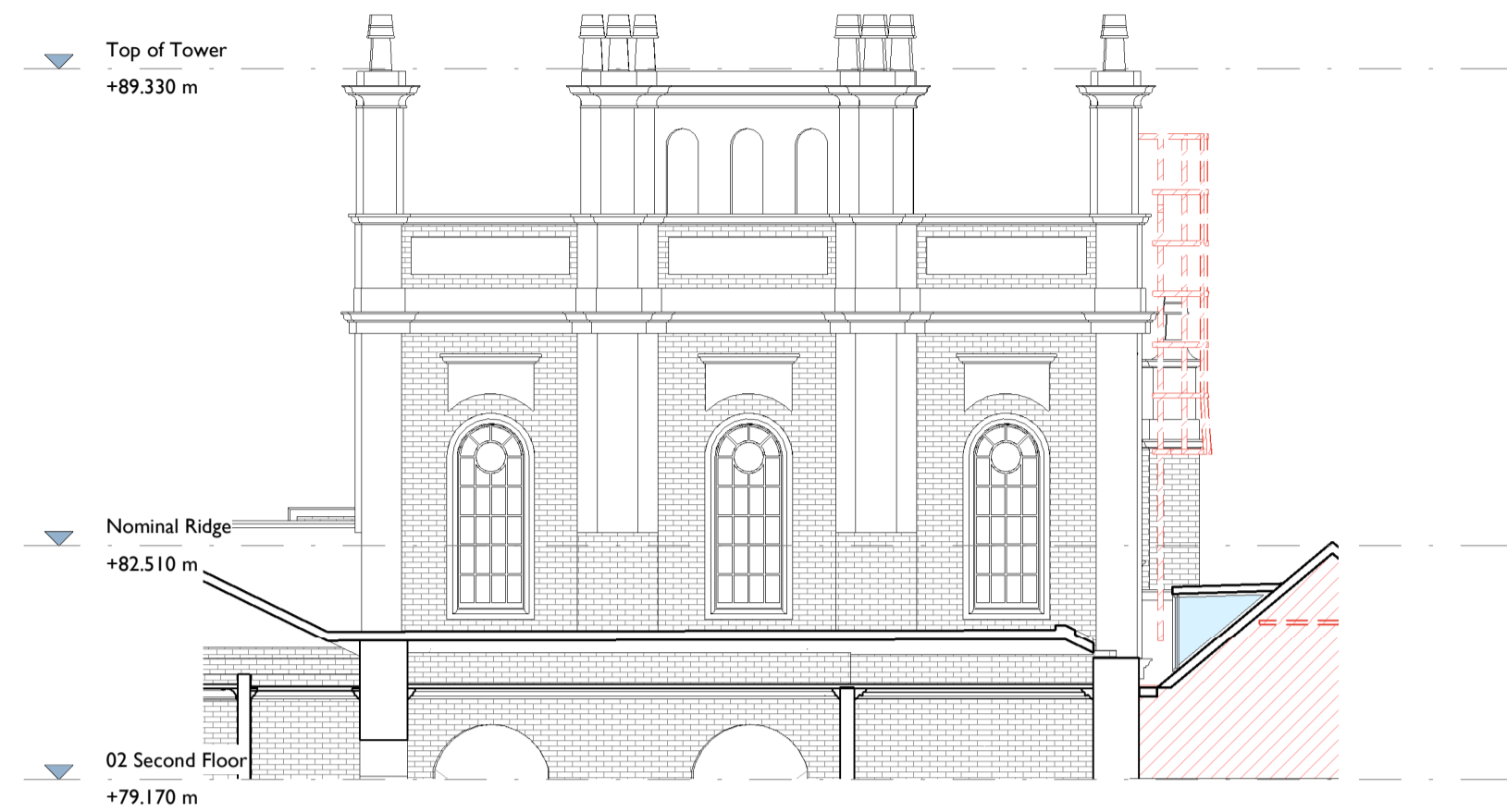
2 Wyatt Wing Elevation 3 (WE3) as Existing Demolition 1017 1 : 100
