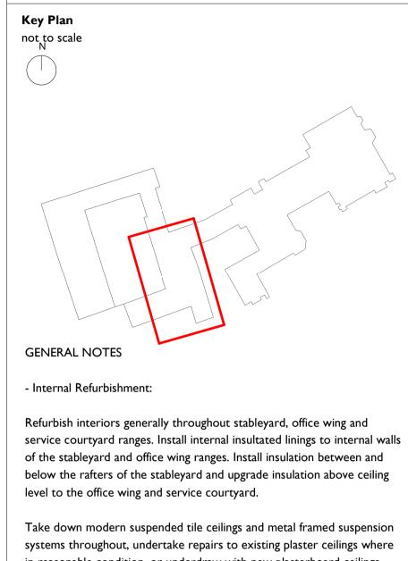
in reasonable condition, or underdraw with new plasterboard ceilings where existing ceilings do not survive / are in poor condition. Where existing floors are modern concrete slabs, excavate, install new
