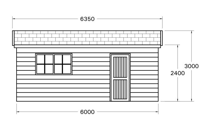
Roof Green Felt Shingles Window Double Glazed. Walls, Slow grown Spruce, thickness 44mm Brown Pressure treated Wood Floor 50mm Concrete slabs laid on sand.
