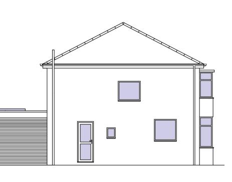
Proposed Side Elevation "A" Scale 1:100
