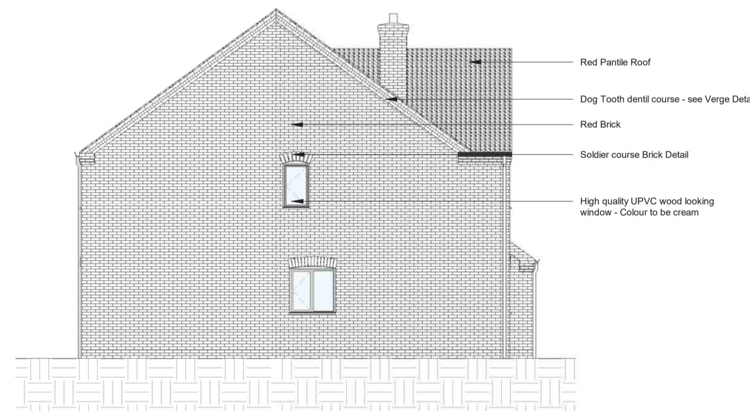
HOUSE 5 - LEFT ELEVATION esc: 1:100
