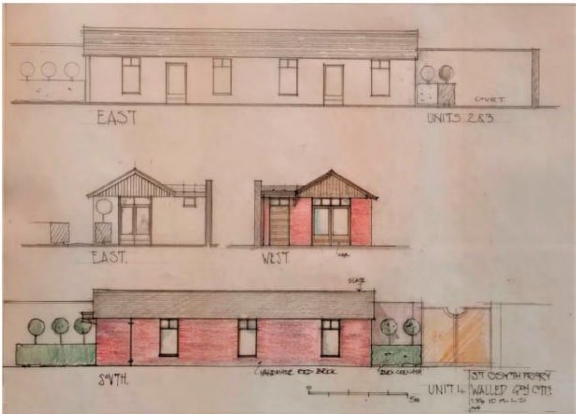
Figure 23b: Typical units - revised design with much lower roofs set well away from walls
