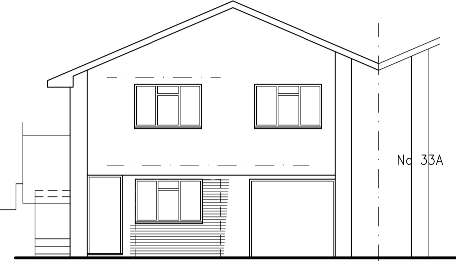
PROPOSED FRONT (SOUTH) ELEVATION New matching window and toothed in matching brickwork
