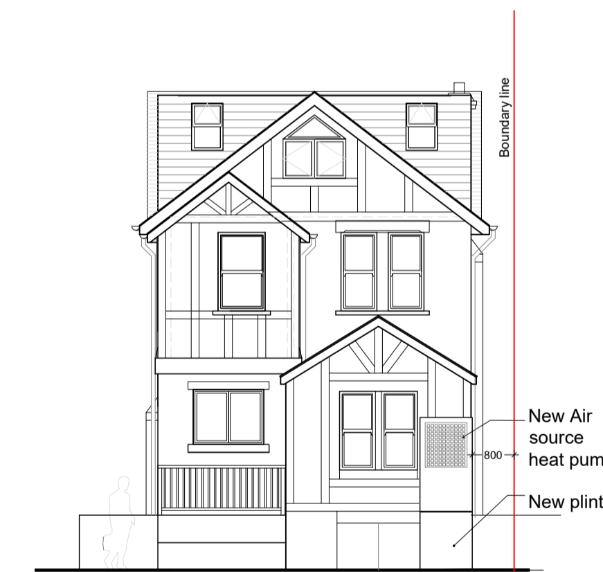
PROPOSED REAR ELEVATION (NORTH) 1:100@A1
