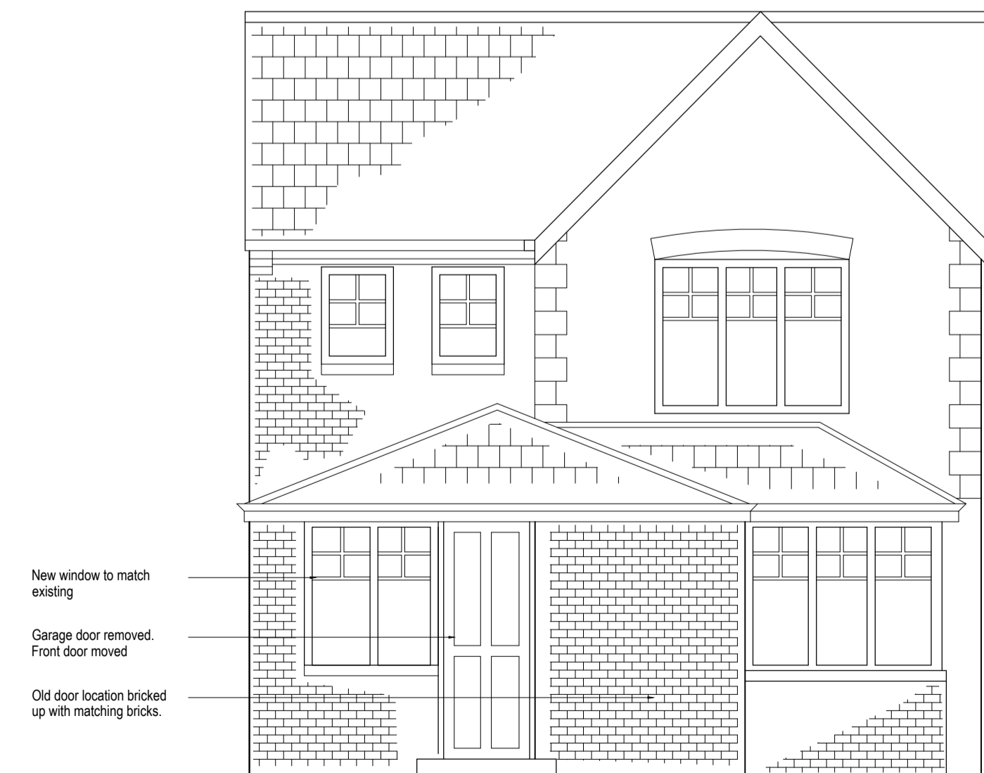
PROPOSED FRONT (NORTH) ELEVATION_SCALE 1:50
