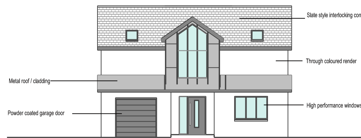
FRONT / SOUTH WEST ELEVATION 1:100
