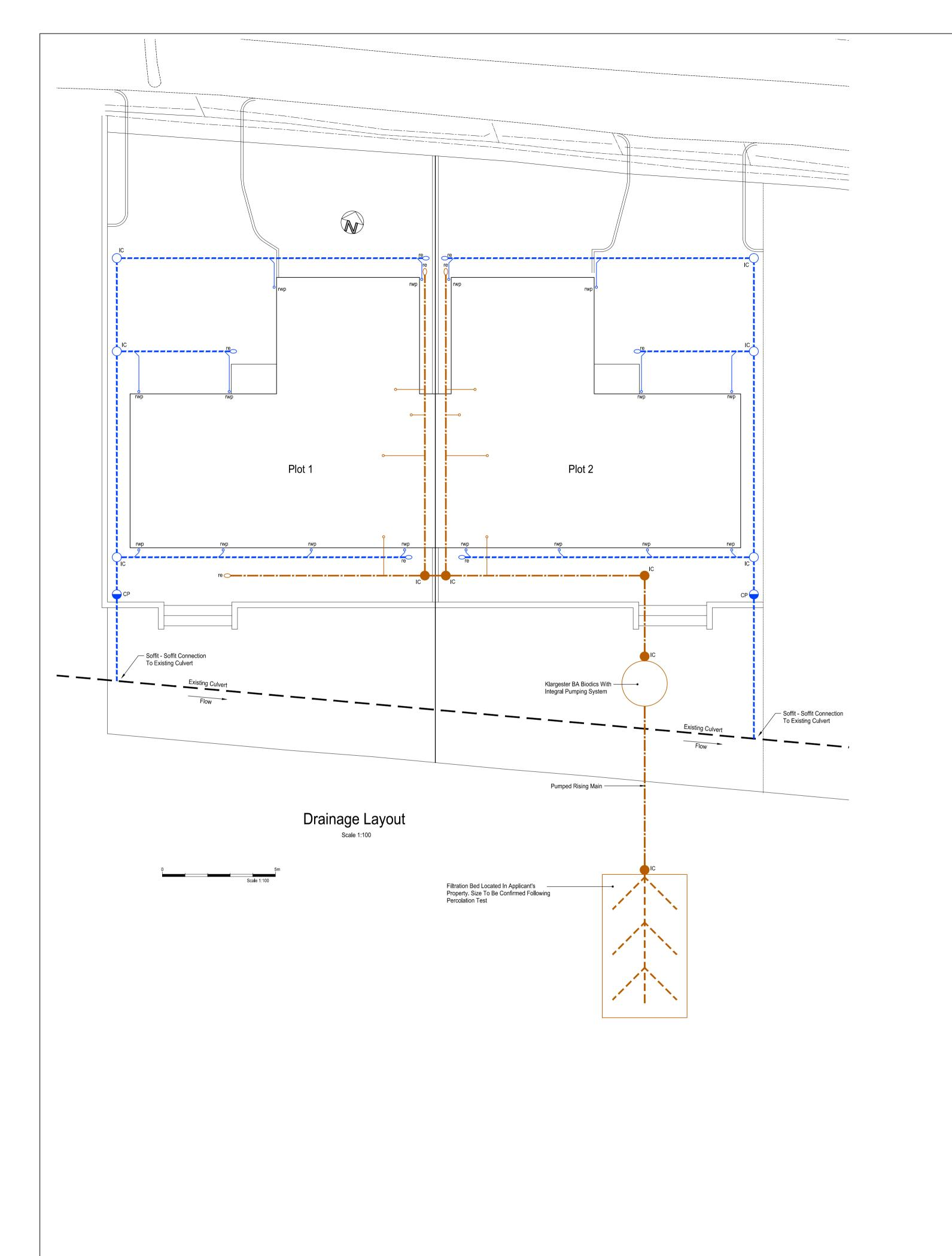
— — — Denotes Ø110mm Foul Water Sewer At Min 1:60 Gradient Denotes Ø110mm Surface Water Sewer At Min 1:100 Gradient
