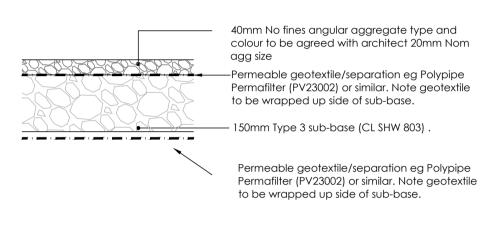
NOTE - GRAVEL WILL MOVE UNDER VEHICLE MANOEUVRES AND REQUIRE OCCASIONAL MAINTENANCE TO RE-ESTABLISH A LEVEL SURFACE NOTE - WHERE LOWER CBR VALUES ARE ENCOUNTERED IT WILL BE NECESSARY TO UNDERTAKE FORMATION IMPROVEMENT BY REMOVAL OF SOFT MATERIAL, PROOF ROLLING, AND ROLLING IN CAPPING LAYER MATERIAL.
