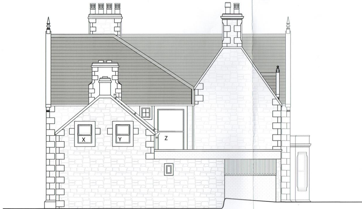
PROPOSED REAR (WEST) ELEVATION 1:50
