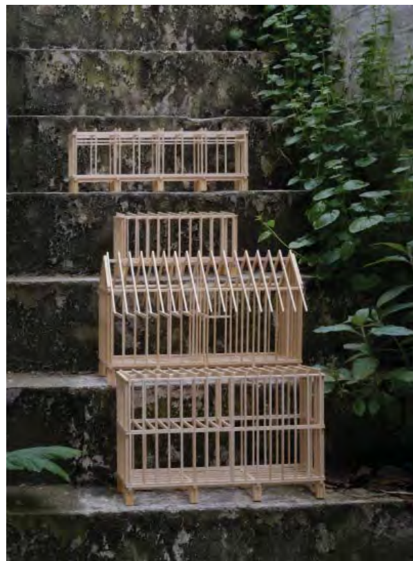
Model studies of timber structures - 1:20
