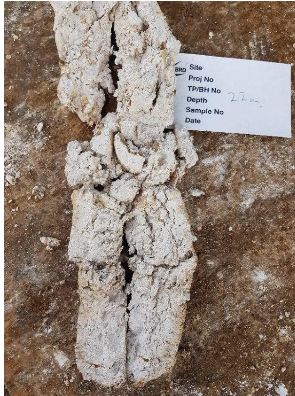
Plate 1: The 22.0m bgl SPT chalk sample with medium spaced discontinuities infilled with brown silt.
