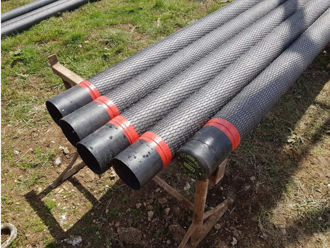
Plate 3: Perforated pipe with 85 micron pore size geotextile wrap with screw in base cap.
