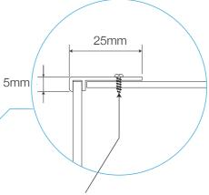
Self tapping screws installed on site to set correct panel alignment, heads painted black to match.
