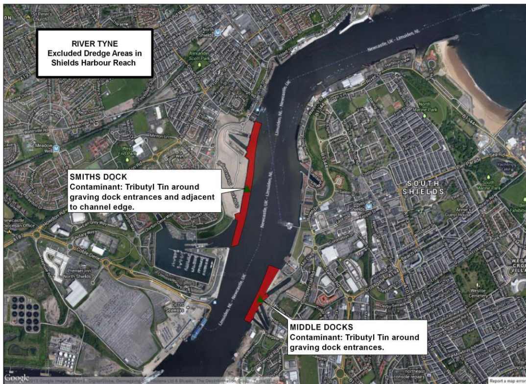
Figure 4.2 Excluded dredge areas in Shields Harbour Reach (as supplied by Port of Tyne Authority)
