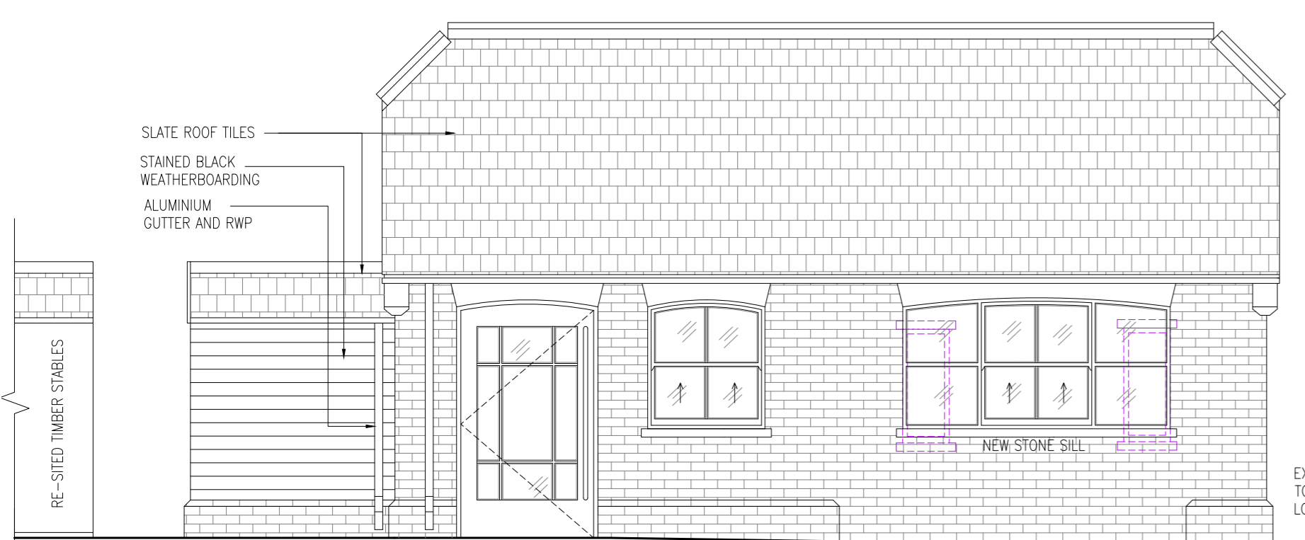
SOUTH WEST ELEVATION
